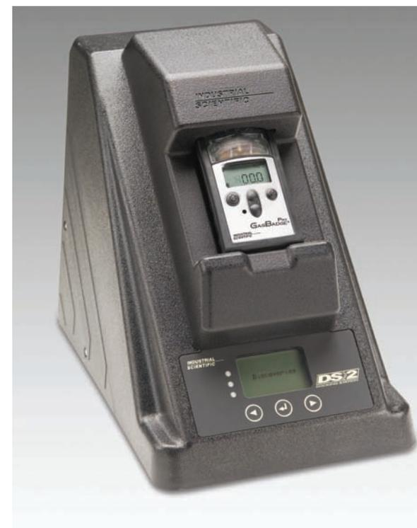
ensure regular instrument calibration is to develop a procedure that includes a schedule for bump testing and full calibration for all gas detectors in a company's fleet.
