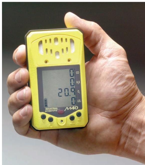
instruments offer quick, push-button calibration with electronic corrections in place of older potentiometer adjustments.
