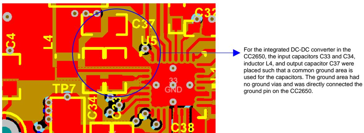
Figure 43. DC-DC Routing Guidelines
