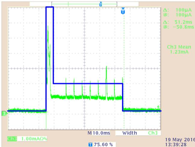
Figure 11. Power Profile During Startup Period
