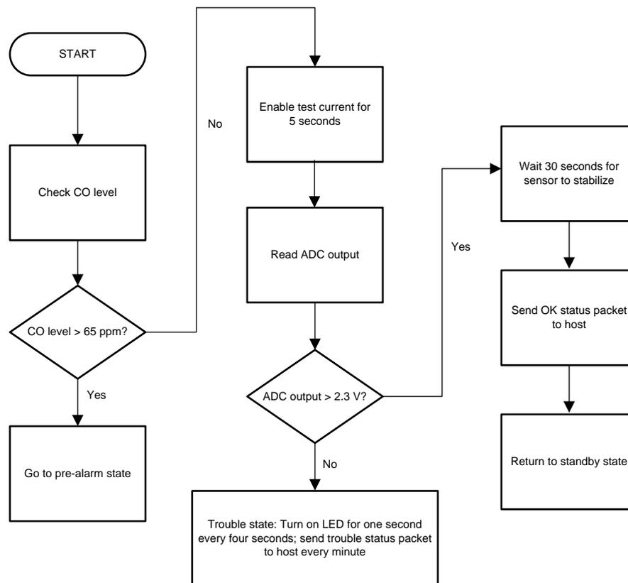
**Figure 14. Sensor Test Procedure**
