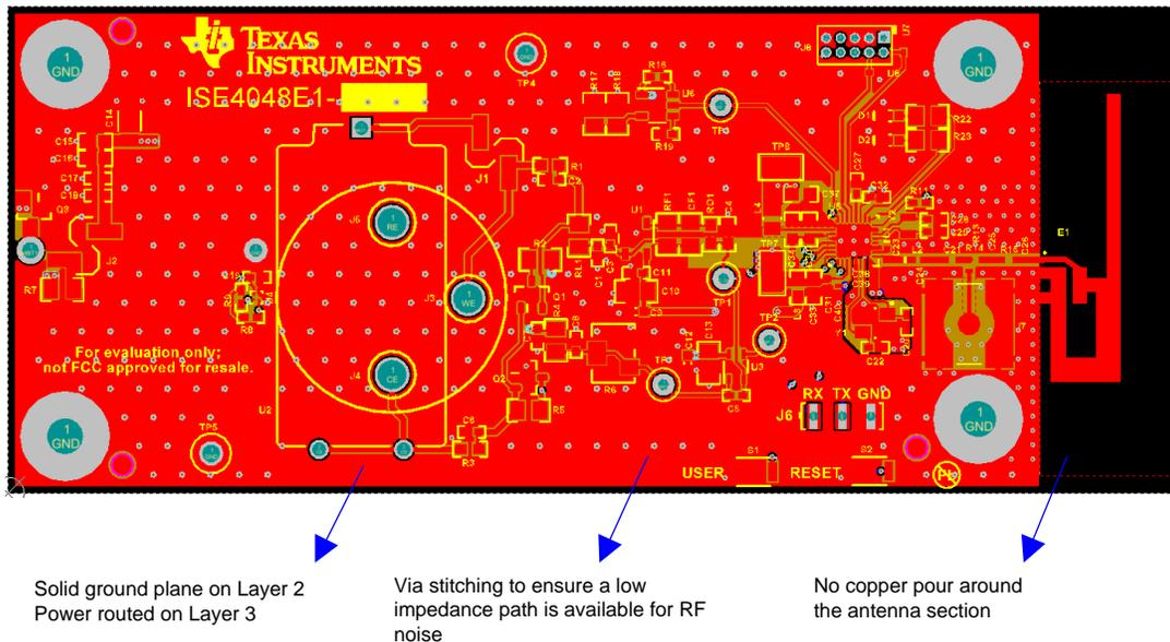
Figure 42. Low-Power Carbon Monoxide Sensor Reference Design Layout Guidelines
