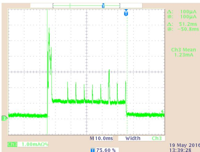
Figure 29. Startup Current at the Beginning of Test State
