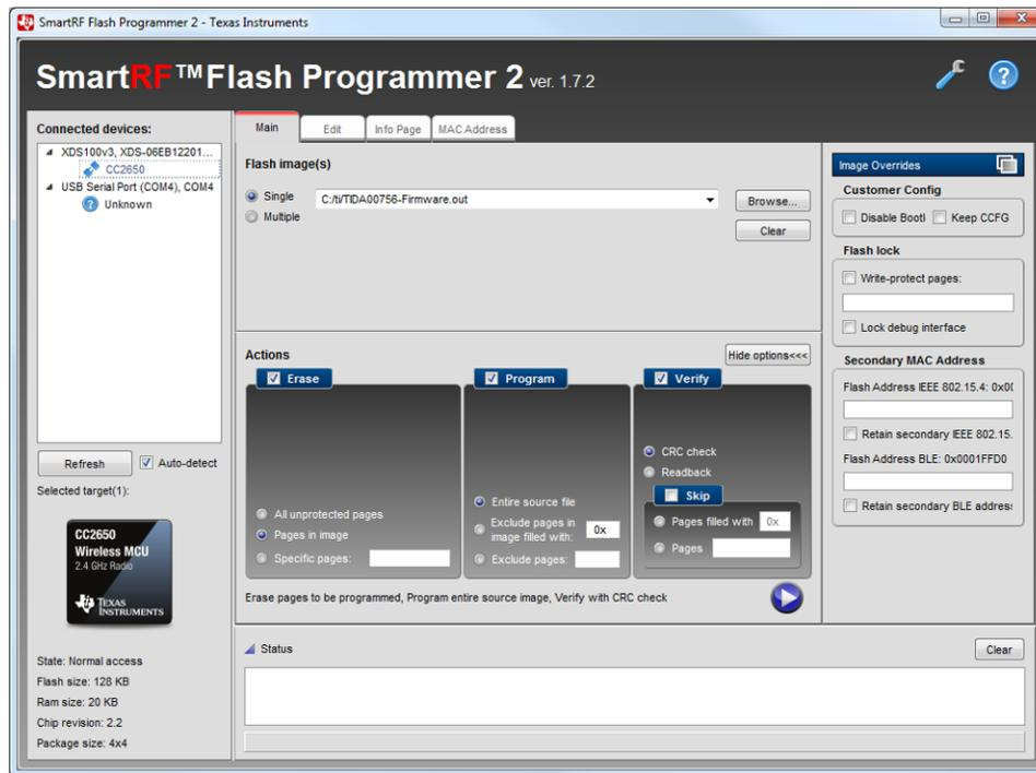
**Figure 18. SmartRF Flash Programmer 2 Configuration**
