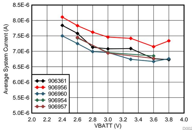
**Figure 31. Pre-Alarm State Current Consumption Across System Voltage**
