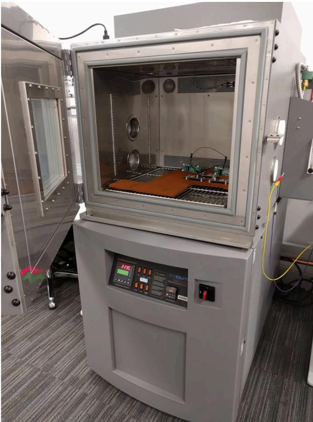
Figure 26. Temperature and Humidity Test Setup
