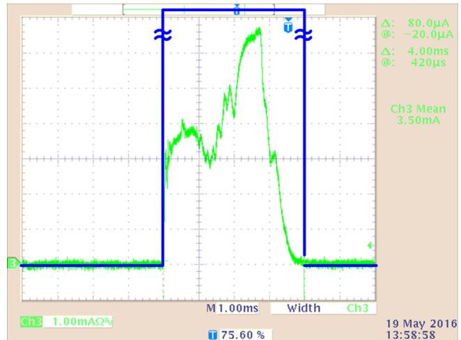
Figure 12. Power Profile During Packet Transmit Period
