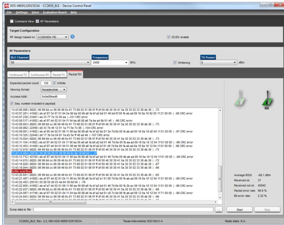
Figure 22. SmartRF Studio Packet Sniffer Recording
