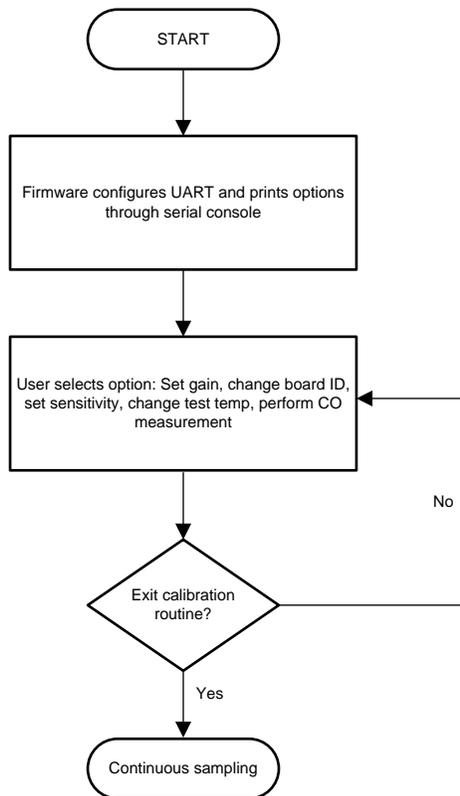
**Figure 15. Calibration Procedure**
