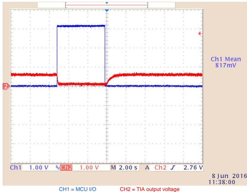
Figure 8. Sensor in Short-Circuit
