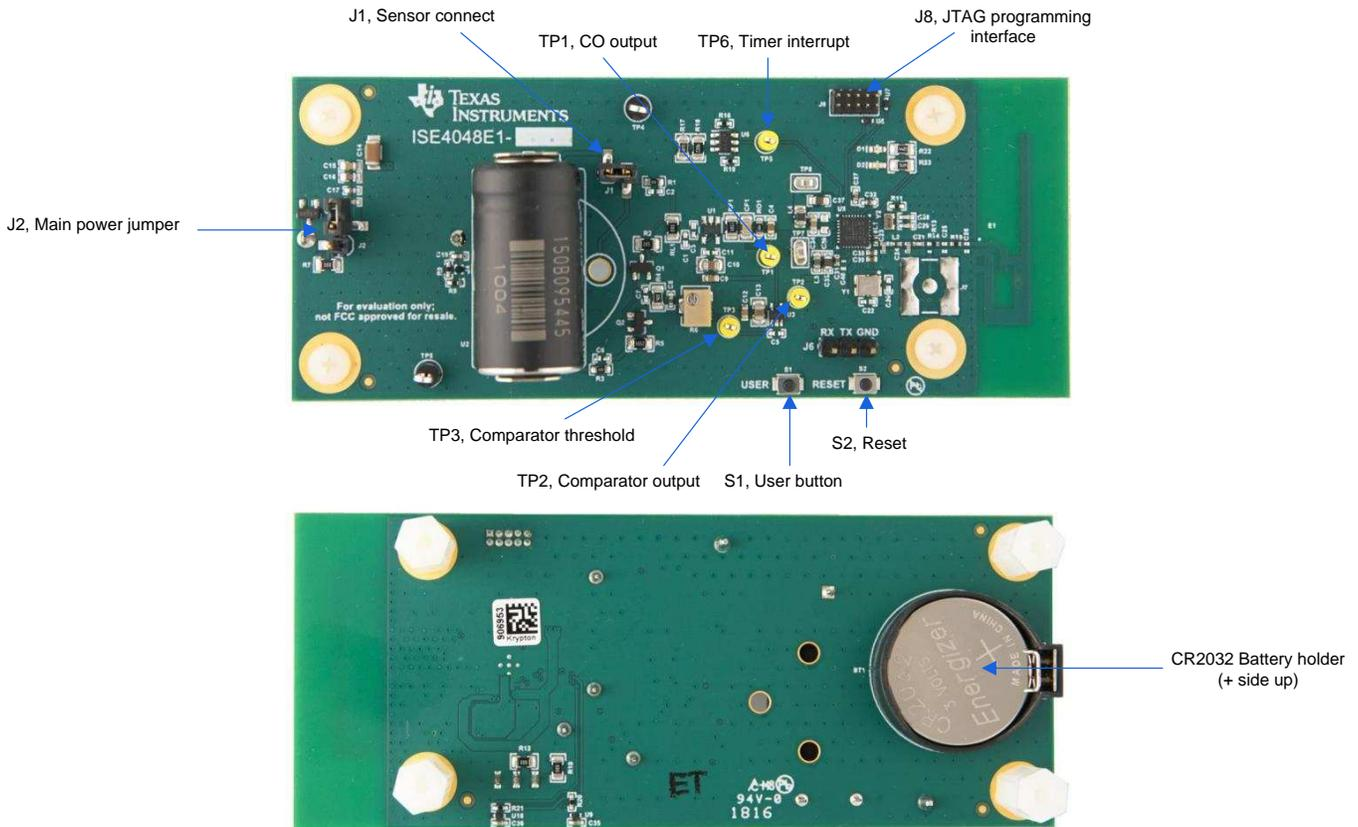
**Figure 16. Low-Power Carbon Monoxide Sensor Reference Design Hardware Description**
