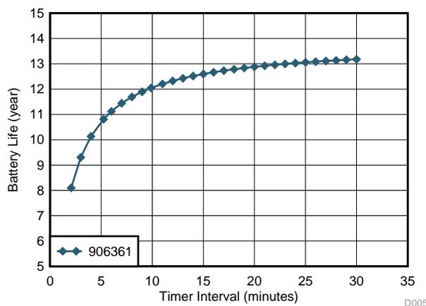
Figure 34. Battery Life versus Timer Interval
