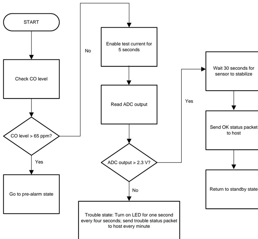
**Figure 14. Sensor Test Procedure**
