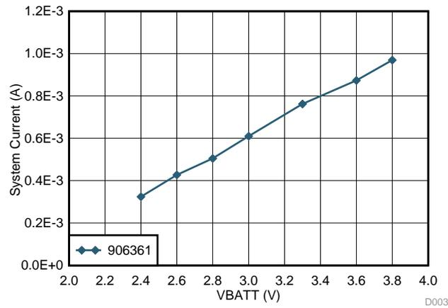
**Figure 32. Alarm State Current Consumption Across System Voltage**
