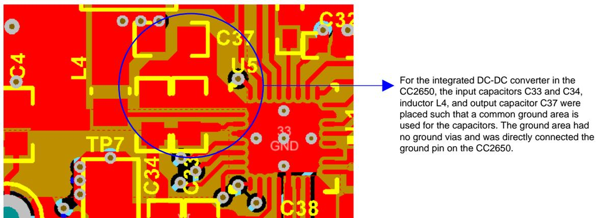
Figure 43. DC-DC Routing Guidelines
