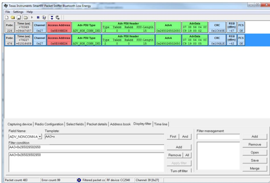
**Figure 21. Packet Sniffer Software, Filtered Recording**
