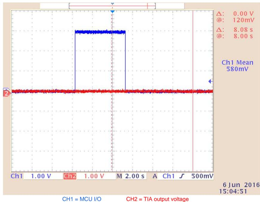
**Figure 7. Sensor in Open-Circuit**
