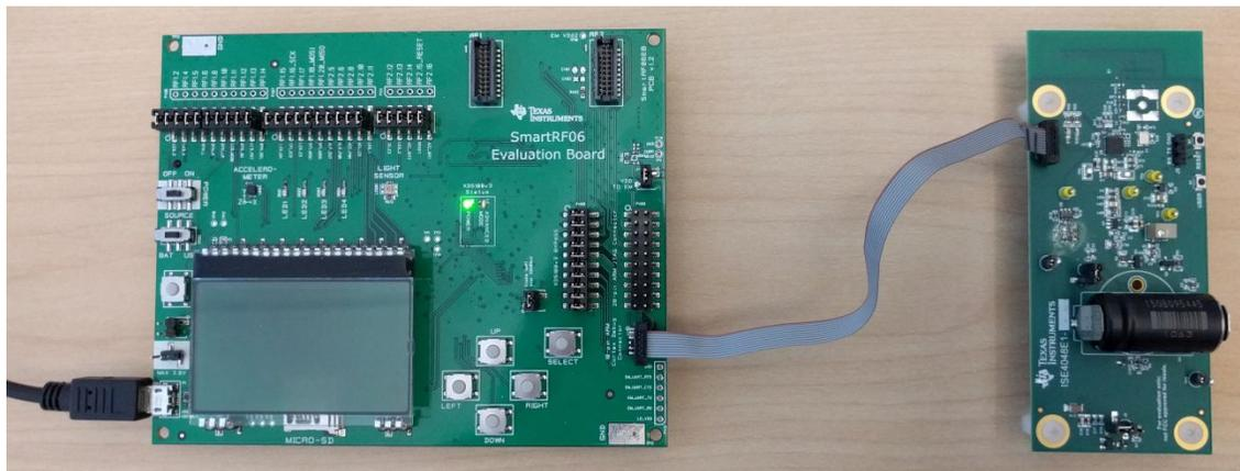
**Figure 17. Connection of SmartRF06 EVM and TI Designs Hardware for Programming and Debugging**
