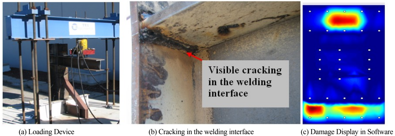
Fig. 10 External Beam-Column Joint Component Testing and Damage Image Display from Acellent ACCESS software
