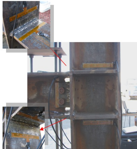
Fig. 9 Smart Patch Sensor Installation for External Beam-column Joint Component
